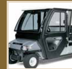
ROPS Cab (Roll Over Protective Structure)
